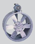
SYMBIOSIS Belt Driven Fans are available from sizes 19" to 75". Fans are driven by belt and pulley arrangement. The motor is located outside the air stream.
